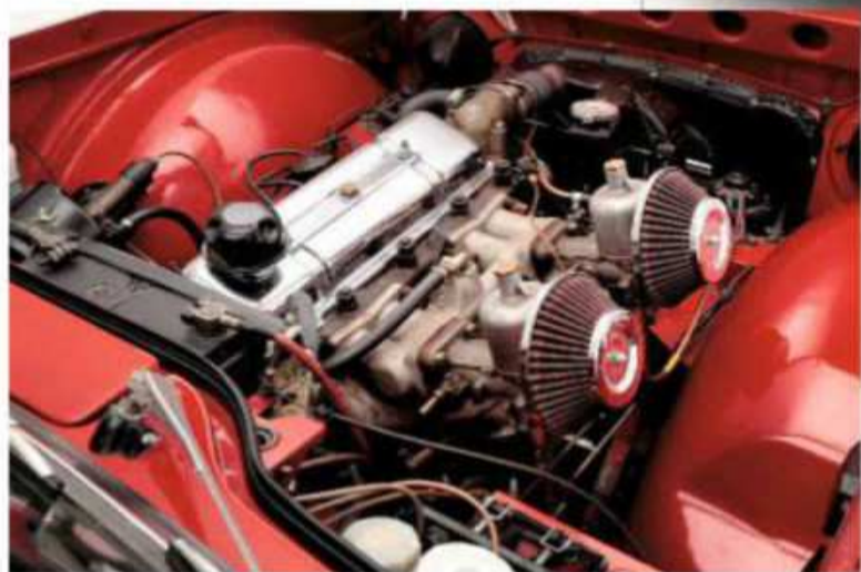
TR4 engine is tough and torquy, but six-cylinder engines are prone to crank thrust washer wear
